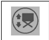
**Debris hopper lifting symbol**
