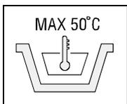
Indicates the maximum temperature of the detergent solution
