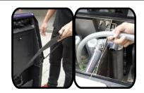
Open the rear cap to access the drain hoses for both the clean & recovery water canks. Once tanks are empty clean both tanks thoroughly. Remove filter bag and rinse with water. Use the tool provided to remove and reattach the filters to clean.
