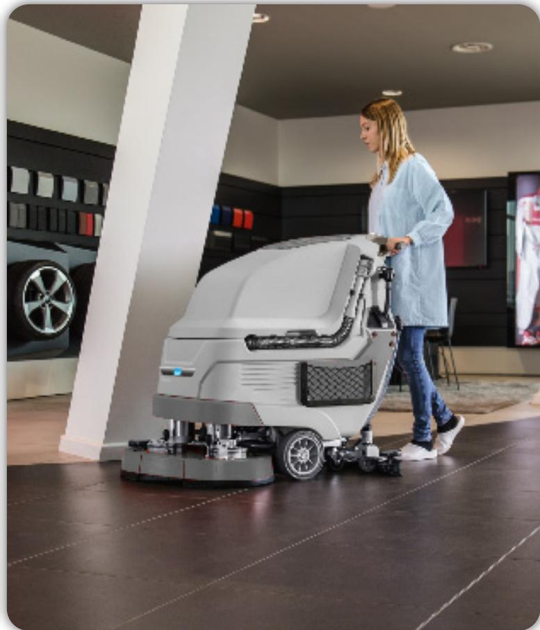
The ICE Scrub 65 D is a battery powered walk behind scrubber dryer with automatic traction and a 65 cm working width.
