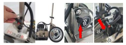
3. Tilt the machine on its rear wheels and rest the handle on the floor
